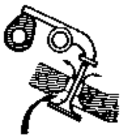
Exhaust valve to be fully opened
