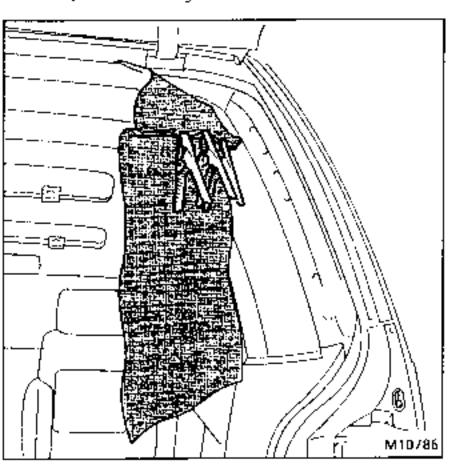
Using a pen, trace the stitching line (over the original holes) to make an easy guide.
