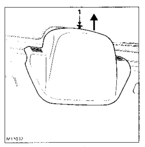
Remove upper mounting (1) from the windscreen wiper casing and pull it upwards to free the lower clips.
