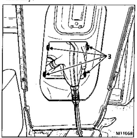
Unclip clips (3) from the gear lever gaiter from the inside.
