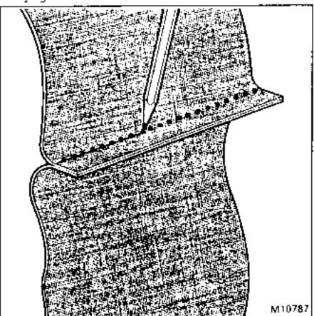
Stitch the trim, aligning the seam over the existing holes of the original seam (using thread the same colour as the trim).
