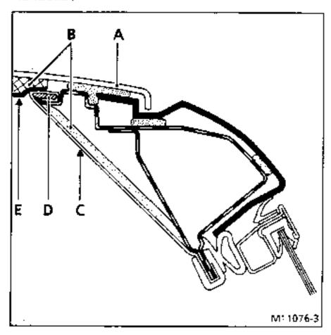
Slide the fabric between the cross members (front, centre, rear) and the head lining using a wooden spatula.
