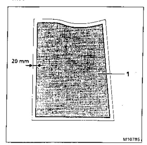
If necessary stick the foam pads back onto the chassis.
