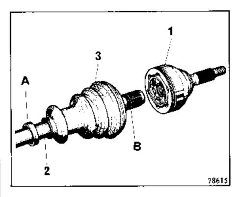
Spread the measured quantity of grease around the gaiter.
