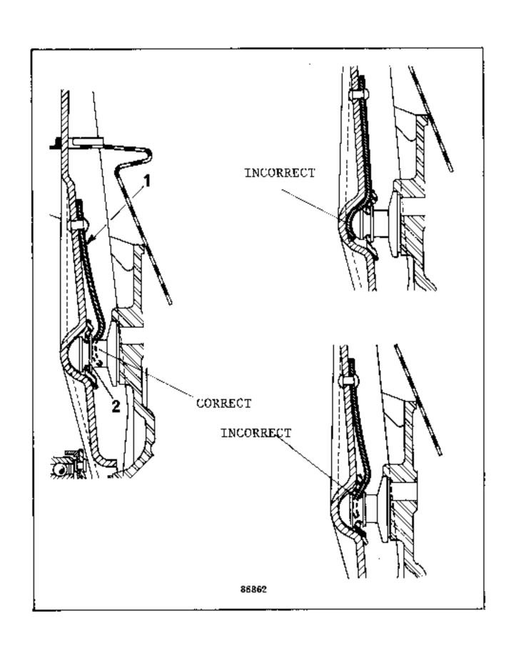
This operation is performed after the gearbox and clutch casing have been removed.
