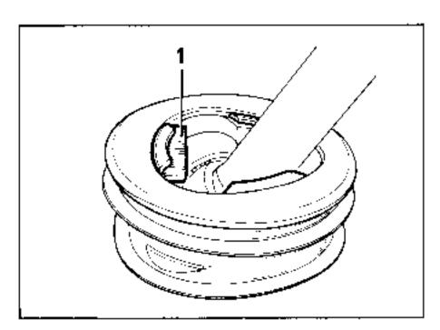
Place the lips on the gaiter in the grooves in the driveshaft and in the casing.
