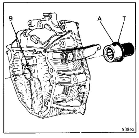
Lubricate the seal before fitting the shaft.
