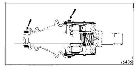
Insert a smooth rod with rounded ends between the bellows and the casing to determine the amount of air remaining in the joint.
