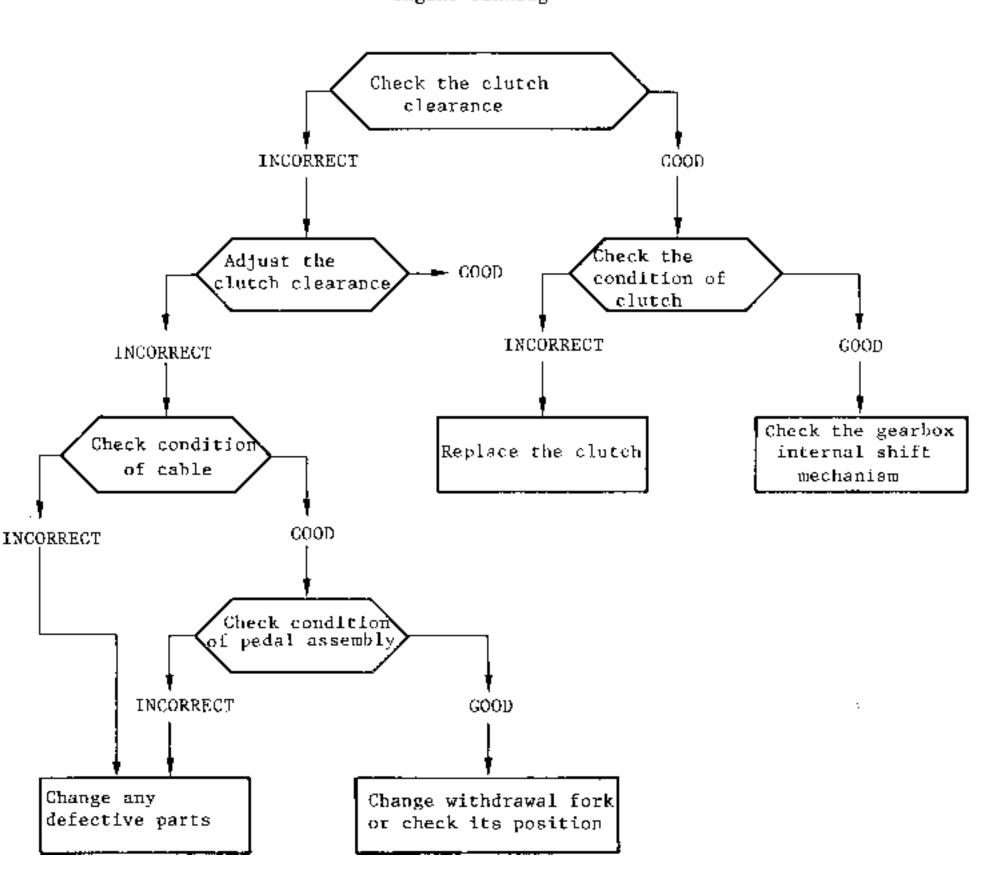
Clutch pedal stiff. Vehicle jerks as the clutch is engaged.
