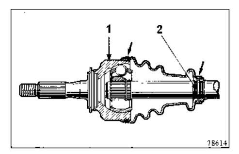
Fit the retaining clips to the gaiter using two rods which are to be made up locally (to the dimensions shown in the drawing).
