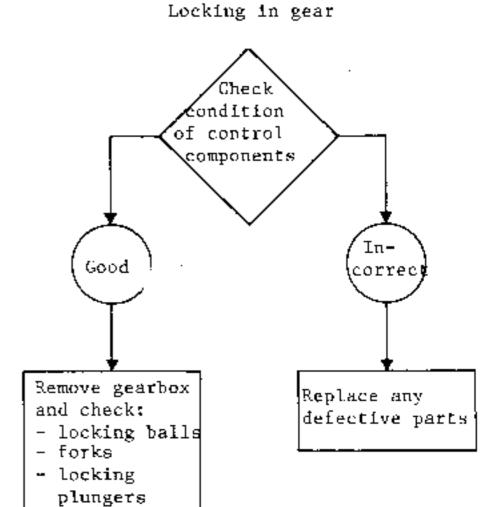
Abnormal noises whilst the vehicle is being driven
