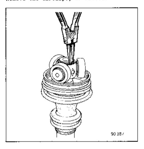
On the press, take out the spider, taking the weight on a stripping extractor.
