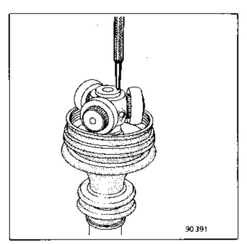
Spread all the grease from the sachet inside the gaiter.
