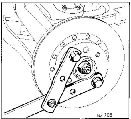
Fit in place the brake callipers, coating the bolts with Loctite FRENBLOC and torque tighten them.
