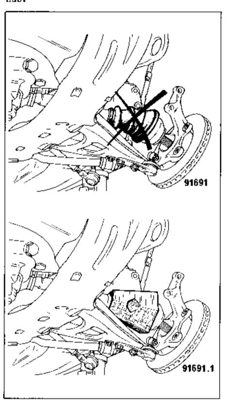
Reconnect the upper ball joint and steering link ball joint and torque tighten the nuts.
