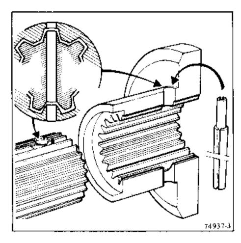
Fit two new spring pins using tool **B.Vi.31.01** and place a few drops of **CAF 4/60 THIXO** in the holes.
