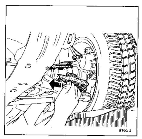
Under no circumstances should a sharp object be used as it could damage the gaiter.
