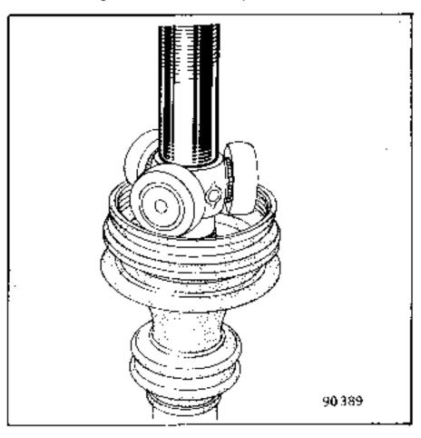
Refit the retaining circlip or pean the metal of the splines onto the driveshaft at points 120° apart.
