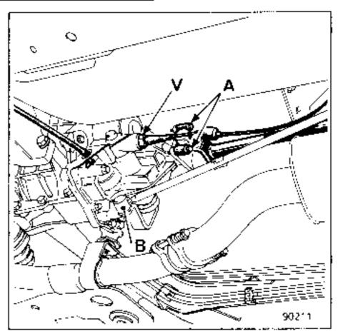
Select 4th gear so that the 5th speed locking ball does not fall into the gear box.
