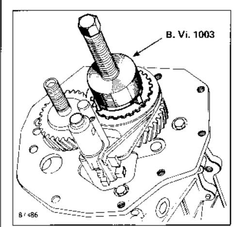
Remove the 5th speed idler gear, bearing and bush.
