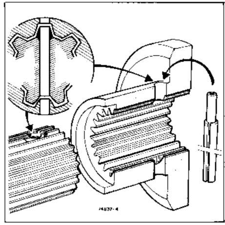
An insert chamfer on the sunwheels makes it easier to fit the new spring pins.
