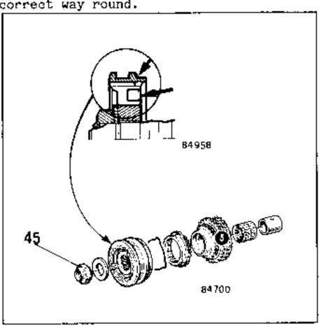
Place the bosses on the synchro ring in the notches in the hub.
