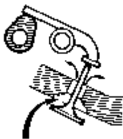
Exhaust valve to be fully opened
